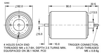
**Outline Note:** The holes at each end are in the same angular position to within  $\pm$  5°; one end must be flexibly connected.
