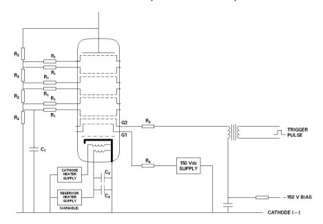
$R_1$  = 470  $\Omega$  2.5 W vitreous enamelled wirewound resistors.
