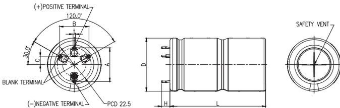
RECOMMENDED PCB PATTERN HOLE SIZE : 2.0(±0.1)mm
