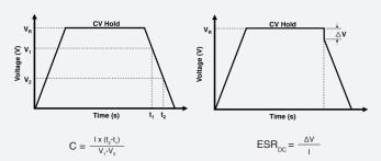
where C is the capacitance (F); I is the absolute value of the discharge current (A);
