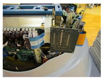
2.4.4 Rotate the Carriage upwards until it is resting on top of the Static portion of the Fixture.
