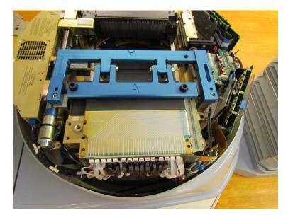
If not, drive the carriage forward or backward with the Service Panel until all holes are aligned. If alignment is not possible using the Service Panel, STOP! Please call AEP Linac!
