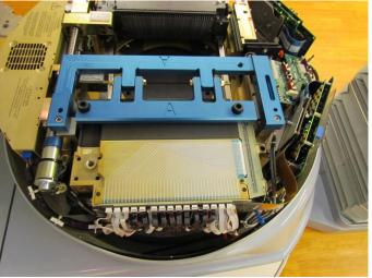
2.3.4 Mount the L-Shaped Handle to MLC Carriage using the far back bolt hole. Use the last 1/2" Socket Cap Head Screw. Verify that there is no contact between Handle and Motor Interconnect.
