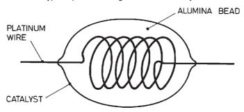
The design has been modified to reduce the amount of power used by the sensor and to make the sensor more resistant to poisoning and mechanical shock. SGX, when known as E2V, was in the forefront of these developments and the current range of pellistors incorporates the design improvements.
