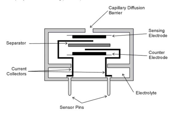
The electrodes need to be kept apart and wetted with an acid electrolyte to allow an ionic current to pass between them. This is done using discs of inert absorbent material or separators. These can be made from materials such as glass fibre.
