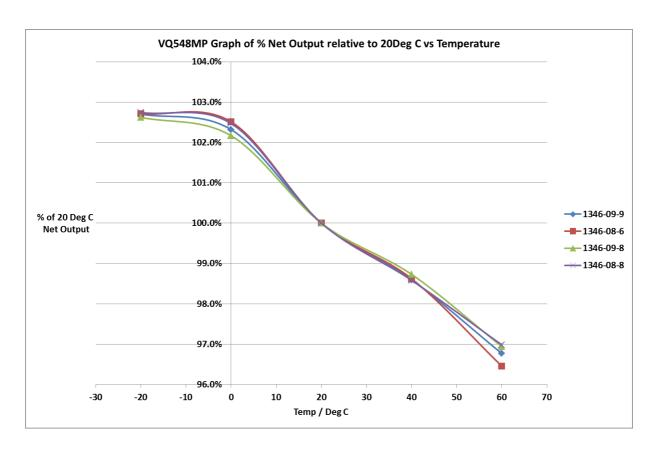
In TC mode, compensation of the zero output is required as the resistance of the compensator will change with temperature unlike that of the resistor. Compensation of the response in Methane is not required as the response curve does not significantly change with temperature. Response curves are independent of temperature.
