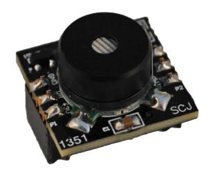
The MP-7217 –TC sensor is a combined pellistor and thermal conductivity sensor designed to measure methane in 2 concentration ranges; 0-100% LEL and 0-100% volume.
