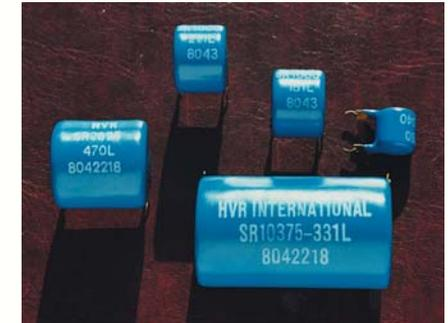
The SR Series of Surge Resistors for PCB mounting are manufactured from a carefully selected mixture of clays, alumina and carbon. After blending, the material is pressed to the required shape and then fired, in a controlled atmosphere, at high temperature.
