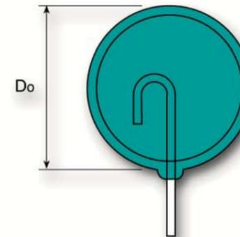
This sintering process produces a Ceramic Carbon Resistor which is 100% active material and therefore of minimum size. The H.V. Resistors for Compact Circuitry range feature radial lead terminations and a high quality epoxy resin coating to improve both dielectric withstand and mechanical robustness.
