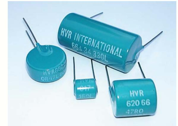
HVR's range of High Voltage Resistors for Compact Circuitry are manufactured from a carefully selected mixture of clays, alumina and carbon. After blending, the material is pressed to the required shape and then fired, in a controlled atmosphere, at high temperature.
