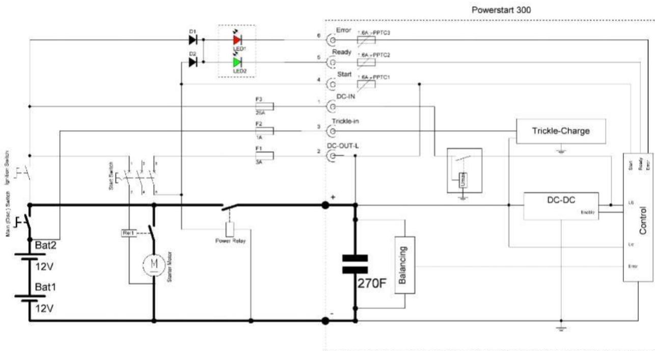
This block diagram is showing a typical (parallel) configuration. Configuration may vary per application. A dedicated start configuration is also possible.
