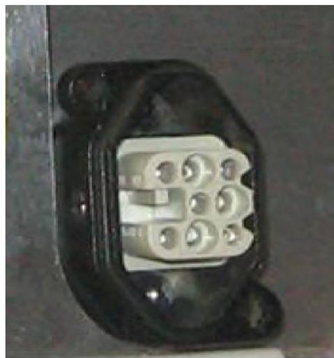
Figure 5: HAN 8D connector on module
