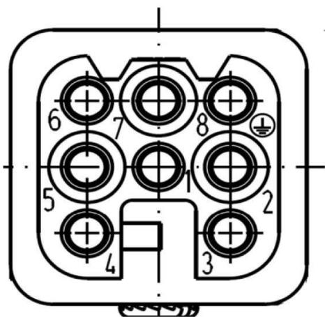
Figure 4: Pin connector HAN 8D (schematic)
