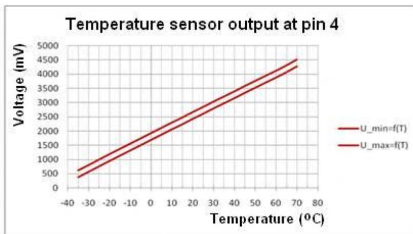
Figure 6: Temperature signal from table; pin 4
