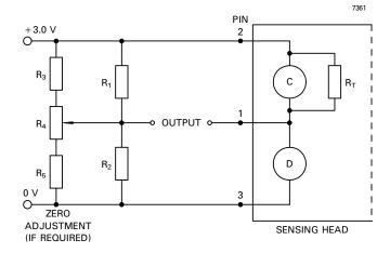
$R_1 = R_2 = 500\Omega$  to 10 k $\Omega$  $R_3 = R_5 \simeq 10R_1$
