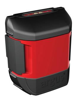
The AA battery pack adds additional flexibility to the Argus® Mi-TIC camera, allowing it to operate for over 4 hours on 7x LR6 AA Alkaline batteries at room temperature. It features a thumb operated latch that allows it to be easily removed and re-attached to the camera.
