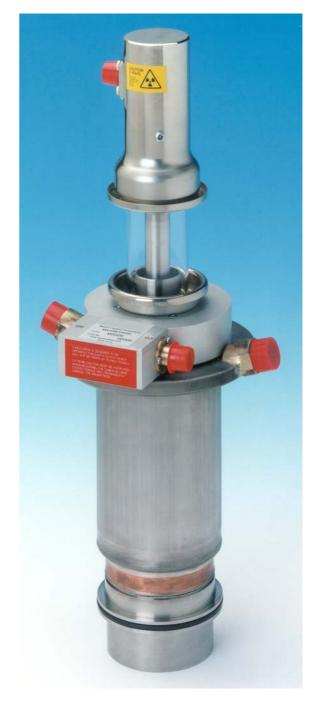
The magnetron output window may be cooled by either high pressure air or an arc suppressant gas such as  $SF_6$ . When the output window is cooled by high pressure air, a flow of not less than 0.085 m³/minute (NTP) into the air inlet at the base of the launching section is required. If  $SF_6$  is used, then no gas flow is required to cool the window. See note 7.
